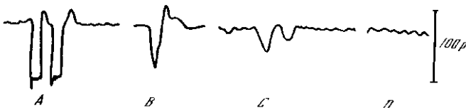
Fig. 14. Amplitude of magnetic signal evoked in the electrical cat-fish by mechanical stimulation vs the distance between magnetometer and aquarium A - 1 cm; B - 22 cm; C - 49 cm; D - 90 cm
